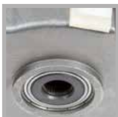
3 Return spring with activation arm coupling
